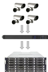
Figure 1: Cameras pass footage to AS72 Server/VMS. AS72 passes footage to storage.
