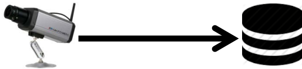
Figure 1 Bosch VMS (BVMS) has direct-camera-to-storage architecture, which by-pass NVR, its OS, and file system
