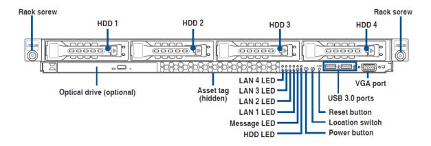
Figure 2: AS175Rv2 Front Panel
