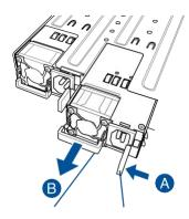
Module lever PSU latch
