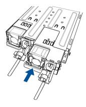
Figure 10: AS175Rv2 PSU Insert / Removal
