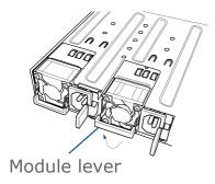
2. Hold the power supply module lever and press the PSU latch, then pull the power supply module out of the system chassis.
