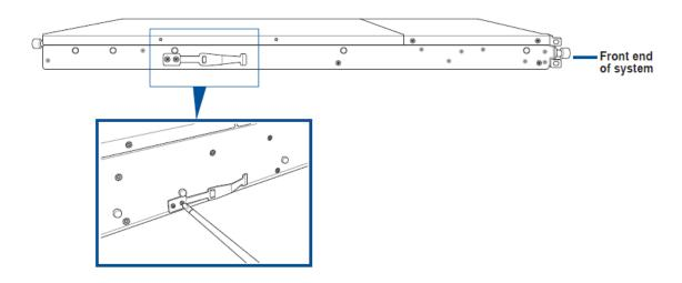
2. Select a desired space and place the appropriate rack rail (left and right) on opposite positions on the rack.
