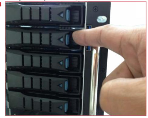
Pull out the HDD tray handle and slide out the HDD tray.
