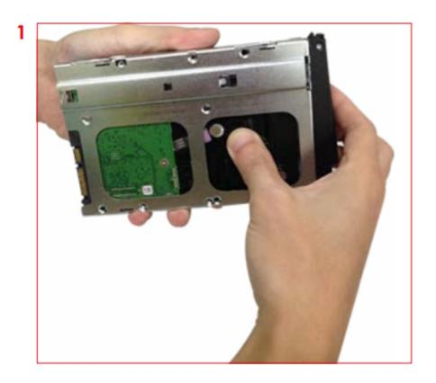
Remove HDD out from HDD tray
