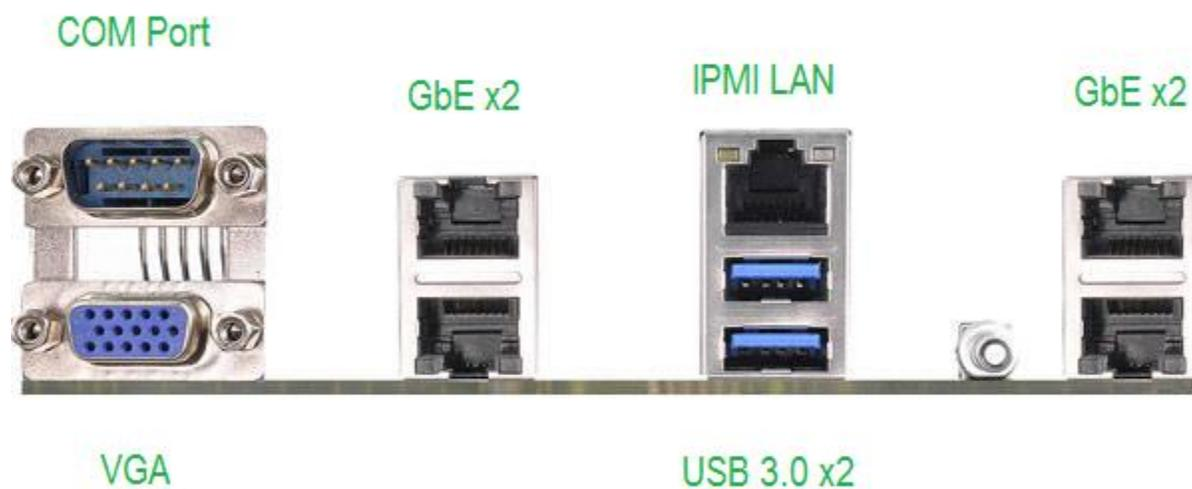
Figure 2-1:AS75 Motherboard Rear I/O
